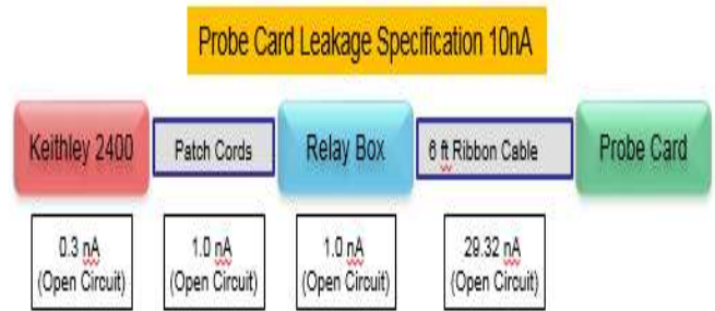
Figure 14: Open-circuit leakage measurements
