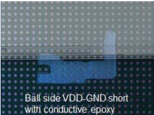
Figure 6. Conductive epoxy is used to short power/ground (VDD-GND) pads on the BGA side.
