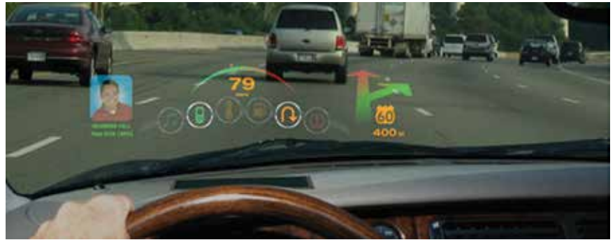
Figure 5. Illustrated above is an example of head-up display (HUD) technology "leveraging night vision, navigation and camera-based sensor technologies to project images produced by ultra violet lasers onto the surface of the windshield." An alternate approach uses TI's DLP ® technology which is fast becoming a new trend in HUD due to its imaging capabilities.
