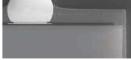
Figure 2a. 5-sided molded WLP (CSPnl™ technology).
