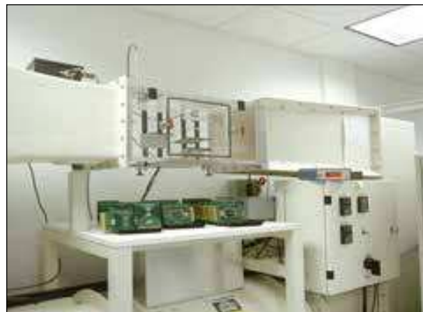
Amkor's closed loop wind tunnel is capable of controlling airflow from 50 to 1600 LPM and air temperature from 18°C to 65°C. The tunnel spatial uniformity of velocity is \pm 1\% of the mean value. The test section is 12" x 12" with a contraction area of 6.5:1.
