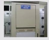
Pressure Cooker Test (Autoclave)
