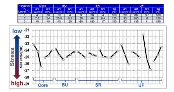
Figure 3. Impact of material properties on UF cracking.
