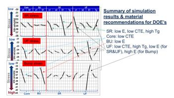
Figure 5. Comparison of impact of material properties on all three mechanisms (SR cracking, UF cracking and bump cracking).
