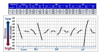
Figure 4. Impact of material properties on chip-interconnect bump cracking.
