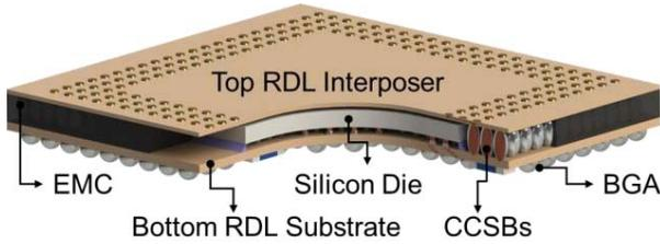
Figure 4. 3D illustration of the RDL-based Interposer PoP.
