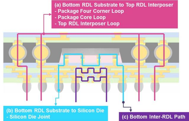
Figure 5. Schematic figure of the three daisy chains' paths.
