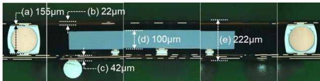
Figure 10. Cross-sectional image: a) CCSB b) Top RDL Interposer c) Bottom RDL Interposer d) Silicon Die and e) Pkg. thickness except BGA
