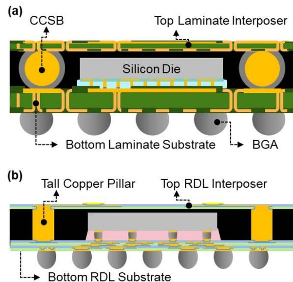
Figure 1. Illustration of Interposer PoP: a) Laminate-based; b) RDL-based.
