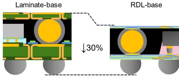
Figure 9. Comparison between a laminated and an RDL-based Interposer PoP
