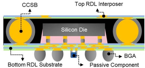
Figure 3. Illustration of RDL-based Interposer PoP with CCSBs
