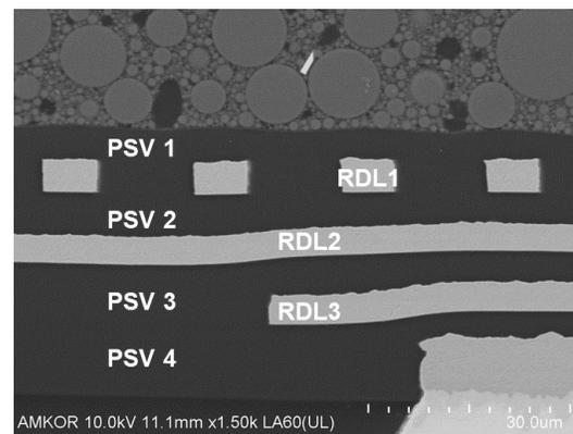
Figure 8. Cross-sectional images of the bottom RDL substrate.
