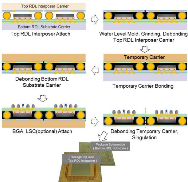
Figure 7. Process flow for RDL-based Interposer PoP with CCSBs.
