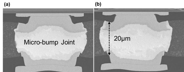
Figure 12. Cross-sectional images of Silicon die micro-bump joint: a) TC 'B' 1000 cycles with Precon L3 and b) after HTS 1000 hrs.
