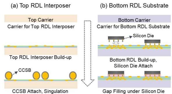
Figure 6. Preparation of (a) top RDL interposer and (b) bottom RDL substrate.
