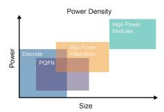
**Figure 2:** Low- to mid-range power applications provide opportunities for innovative integrated power packaging that overlaps the discrete and PQFN spaces.
