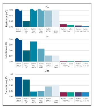
**Figure 7:** Simulated comparison of  $R_{DS}$ ,  $L_{DS}$  and  $C_{iss}$  for the PowerCSP<sup>TM</sup> (PCSP) design to different versions of eD2PAK, TOLL and LFPAK packages.
