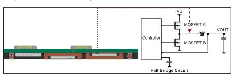
Figure 8: The PowerCSP™ design methodology can be used to construct a power module package.
