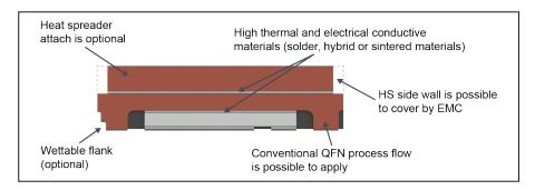
Figure 3: The first implementation of PowerCSP™ technology shows its flexibility and many construction options.
