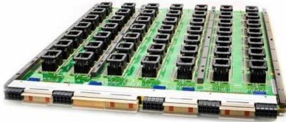
Figure 8: Burn-in Board with Sockets, PCB, Frame and Signal, Power and Ground Connectors. Source: KES Systems [5].
