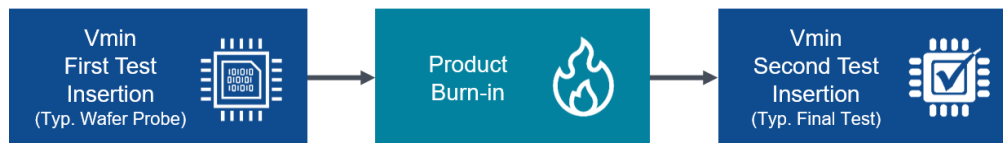
Figure 3: Measure of Burn-in: V_{min} Degradation.
